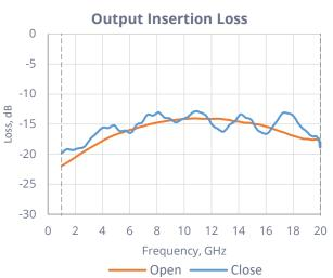
GaAs MMIC, Wide Band, Reflective, SPDT Switch, 0.1 – 20 GHz
